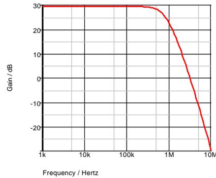
Fig. 14-30: Frequency response of the class AB amplifier.
